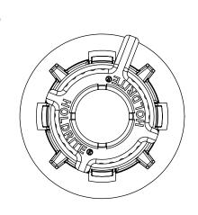
The HOLDRITE® LOCK-n-LOAD™ #701 is a clamp that mounts into our #103, #709, #110-R or #721 Series Bracket. This clamp requires no hardware to install and is designed to firmly grip fixture stub-outs such as bullets or similar 1/2" CTS tubing. The HOLDRITE LOCK-n-LOAD #701 is for use with PEXRITE Brackets only.
